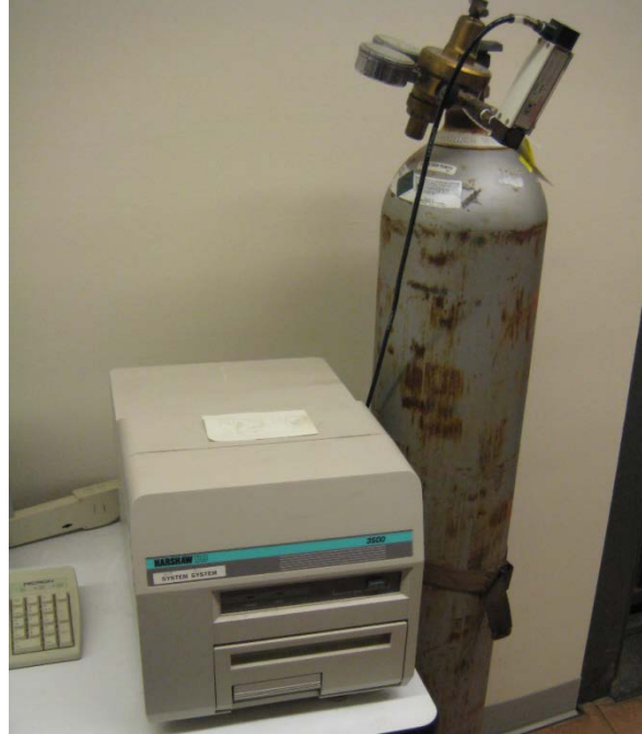
Figure 3-8: The system setup of the Harshaw Model 3500 Manual TLD in building 470.
