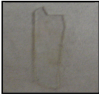
Figure 1-3: This sample was purchased from Newlight. Little is known about its growth technique. It was originally a part of a larger disc. The sample was extremely clear and transparent prior to irradiation.
