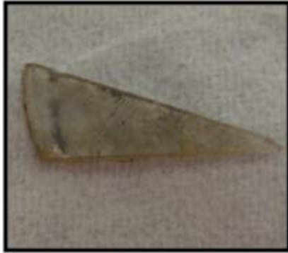
Figure 1-4: This copper doped sample was grown in the Ukraine and received in the 2 nd batch that AFIT received. It is doped with 0.015% Cu and was generally clear prior to irradiation.
